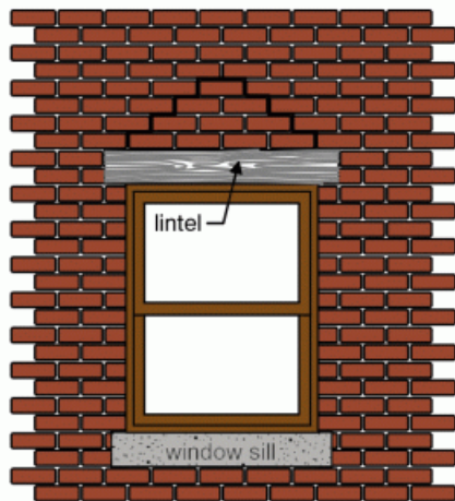
cracking caused by deterioration of wood lintel
